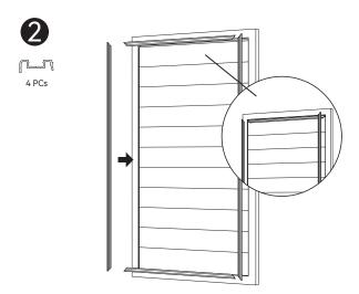
Start by installing the short edge covers on the top and bottom, followed by the long edge covers on the sides. Arch the cover slightly to insert both ends first, then use a rubber mallet to tap from the ends toward the center for a secure fit.
