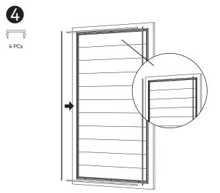
Start by installing the short cover tops on the top and bottom, followed by the long cover tops on the sides. Arch the cover slightly to insert both ends first, then use a rubber mallet to tap from the ends toward the center for a secure fit.
