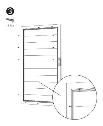
Start by installing the short cover tops on the top and bottom, followed by the long cover tops on the sides. Arch the cover slightly to insert both ends first, then use a rubber mallet to tap from the ends toward the center for a secure fit.
