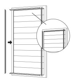
Start by installing the short edge covers on the top and bottom, followed by the long edge covers on the sides. Arch the cover slightly to insert both ends first, then use a rubber mallet to tap from the ends toward the center for a secure fit.
