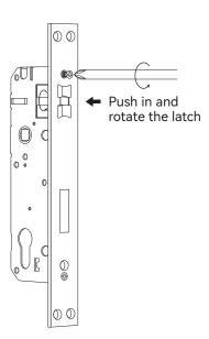
(Optional) Switch the latch according to door opening direction.
