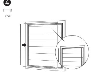
Start by inserting both ends first, then use a rubber mallet to tap from the ends toward the center for a secure fit.
