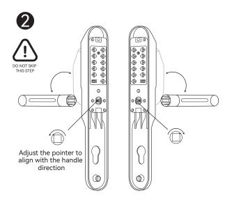
Adjust the handle direction according to the door opening direction
